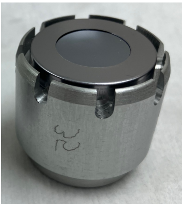
GaAs wafer on Moly puck # 35 ear up
