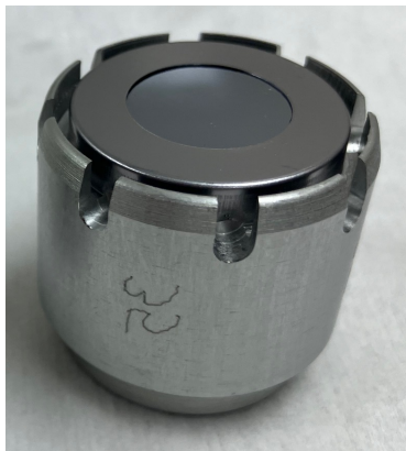
GaAs wafer on Moly puck # 35 ear up
