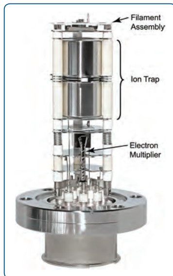
VQM Ion Trap Mass Spectrometer Gauge
