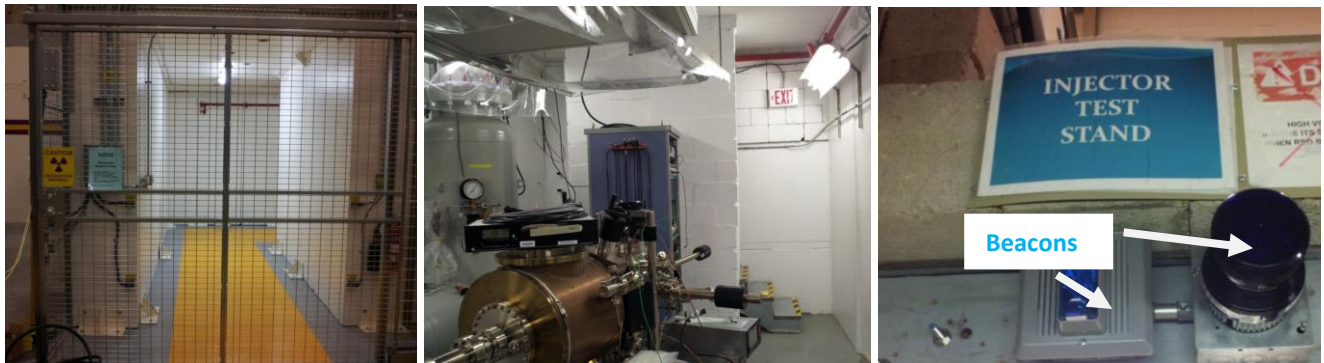
Figure 11 (Left) Main entrance/exit through the labyrinth of UITSF, (Middle) Secondary entrance/exit from the southern-most location of the keV section in Cave 1. Both doors have Personnel Safety System interlocks and emergency exit switches on the nearby walls, (Right) Beacons exist at both entrance/exit ways
