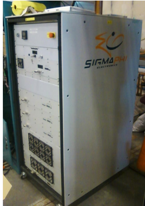
Figure 1: (left) the normal-conducting copper-cavity 748.5 MHz buncher installed on the UITF keV beamline, and (right) the 7 kW solid state amplifier located above Cave 1 near the electronics racks.
