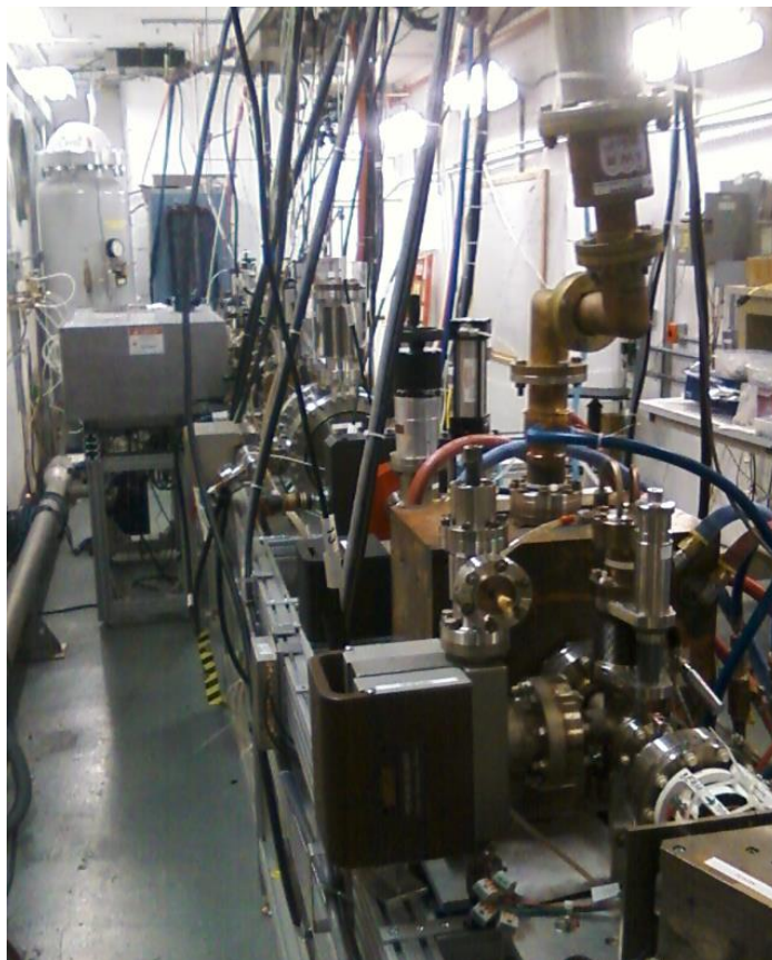
Figure 7: Photograph of the buncher installed on the keV beamline at UITF, looking toward the photogun.
