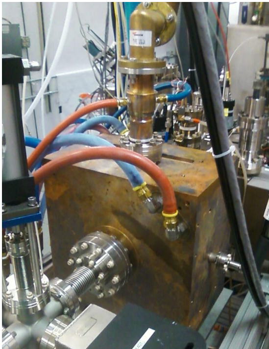
Figure 1: (left) the normal-conducting copper-cavity 748.5 MHz buncher installed on the UITF keV beamline, and (right) the 7 kW solid state amplifier located above Cave 1 near the electronics racks.
