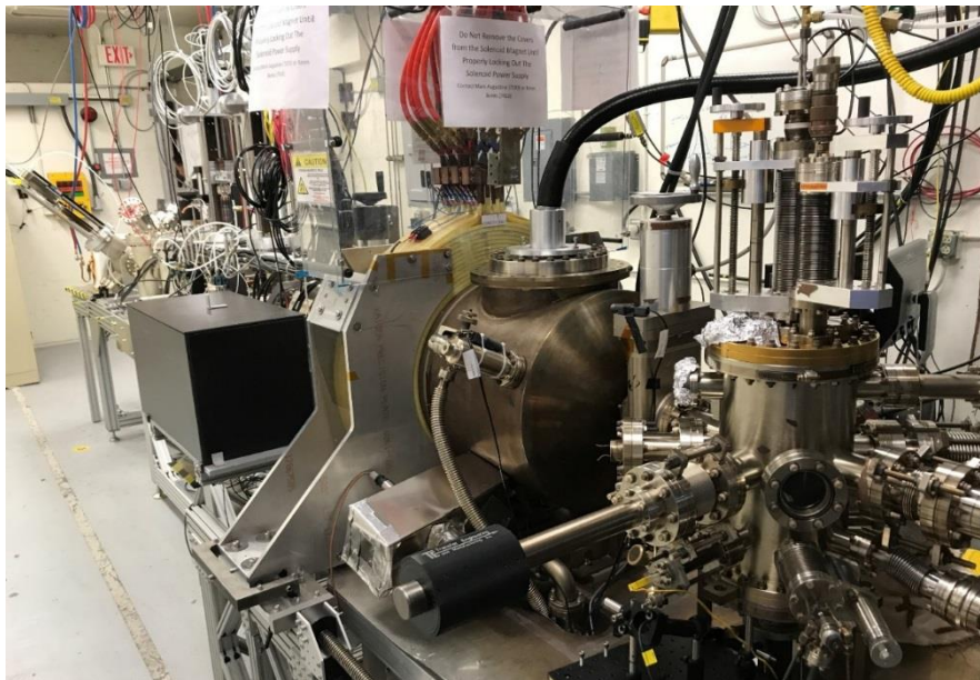
Magnetized photogun and beamline at the GTS
