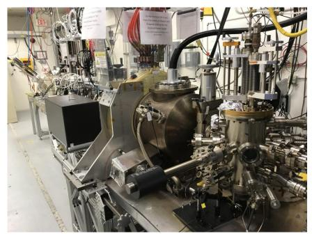
Measuring beam mechanical angular momentum (beam magnetization) using slit and viewer screen method with 1511 G at photocathode
