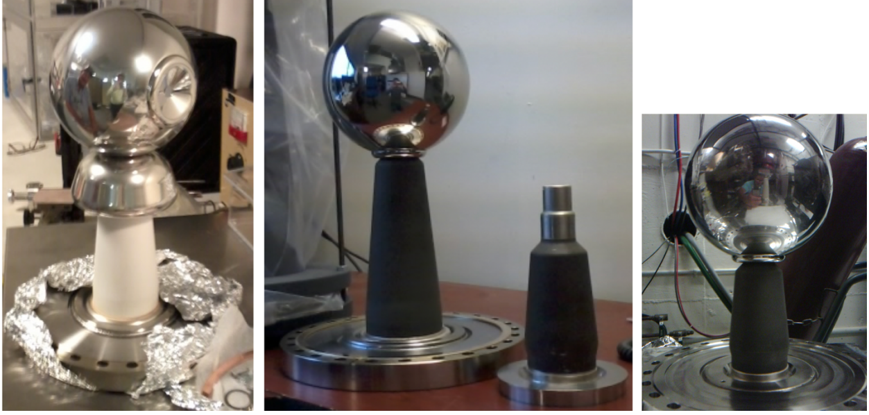
Figure 4. Inverted insulators and electrode configurations studied at JLab. Left: Pure alumina large R30 insulator (7.5" tall) with spherical and screening electrode. Center: Doped alumina large R30 insulator with spherical electrode only and welded to 10" CF flange, next to small R28 doped alumina insulator (4.5" tall). Right: Doped alumina R28 small insulator with spherical electrode only and welded to 10" CF flange.
