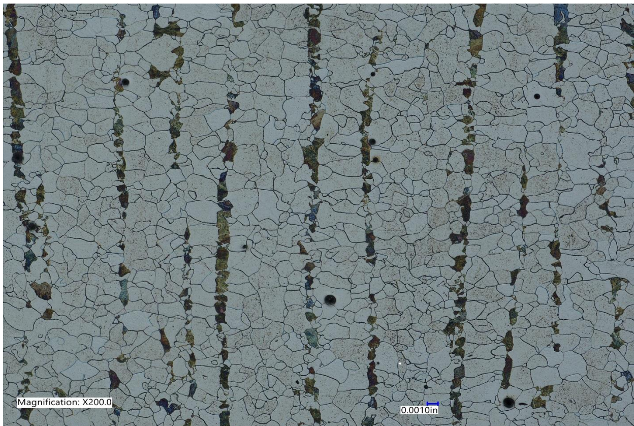
Core microstructure 200x: CC
