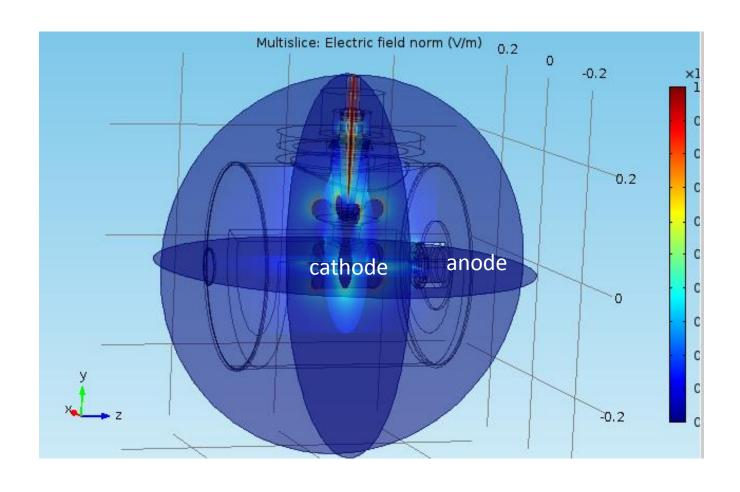
• This image shows the electric field norm |E| in MV/m as color intensity. The coordinate system is as shown for all plots and images the origin is at the center of the cathode electrode. (The anode is at the right )
