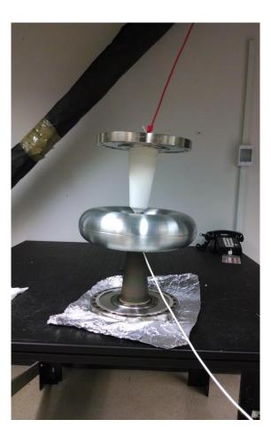
Test of pure Alumina ceramic. Apparatus is flipped.
