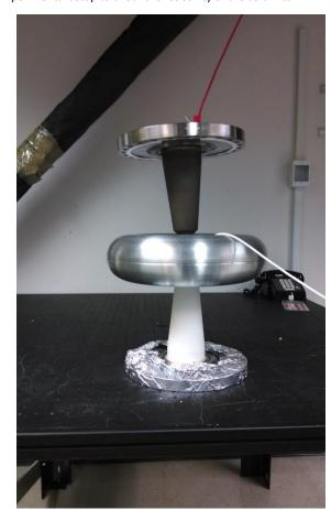
A current limited (<5mA) Bertan 6KV power supply is used to bias the mid point of the ceramic stack.
