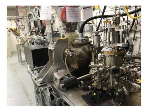
Measuring beam mechanical angular momentum (beam magnetization) using slit and viewer screen method with 1450 G at photocathode
