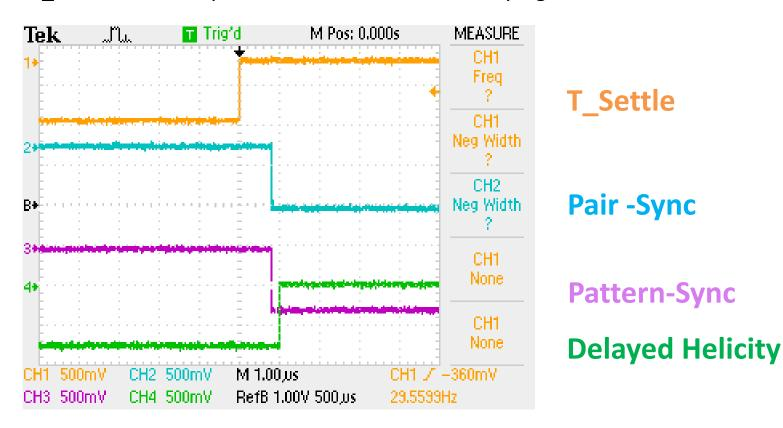
$\Delta T(nT\_Settle - PairSync) = 0.94 \mu s$
