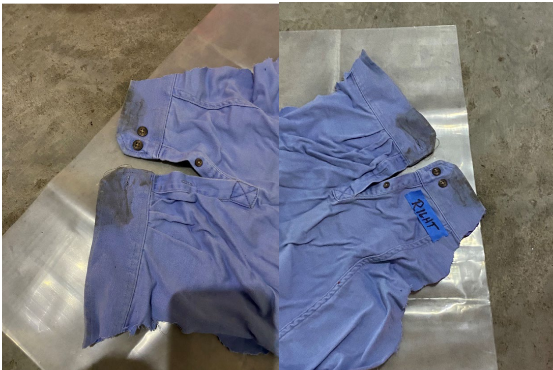
Figure F-6: Left and Right sleeve cuffs on the arc-rated shirt showing either dirt or possible soot and slight water marks but was inconclusive.
