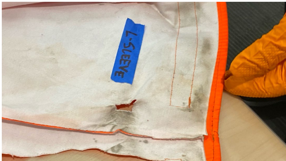
Figure F-11: Inside of left sleeve cuff there is a small open hole with either dirt or minor soot deposits. Possible arcing point.
