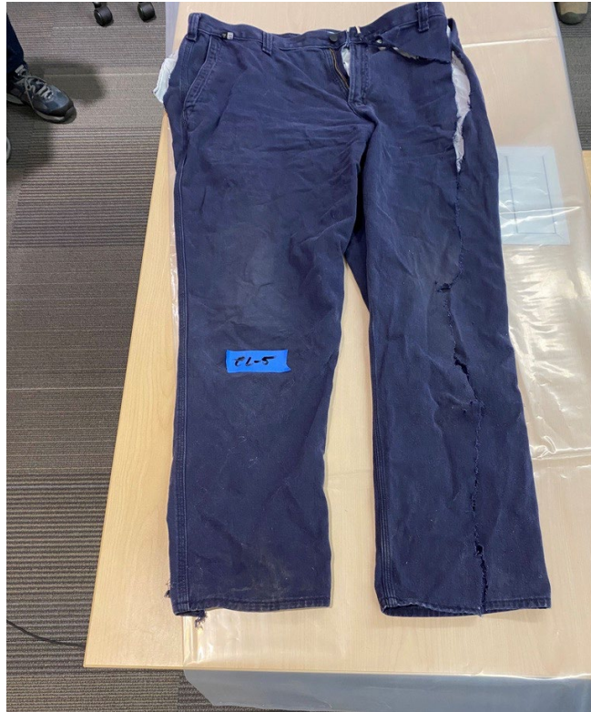
Figure F-8: Front of arc-rated pants showing some dirt but no sign of arc flash burning.
