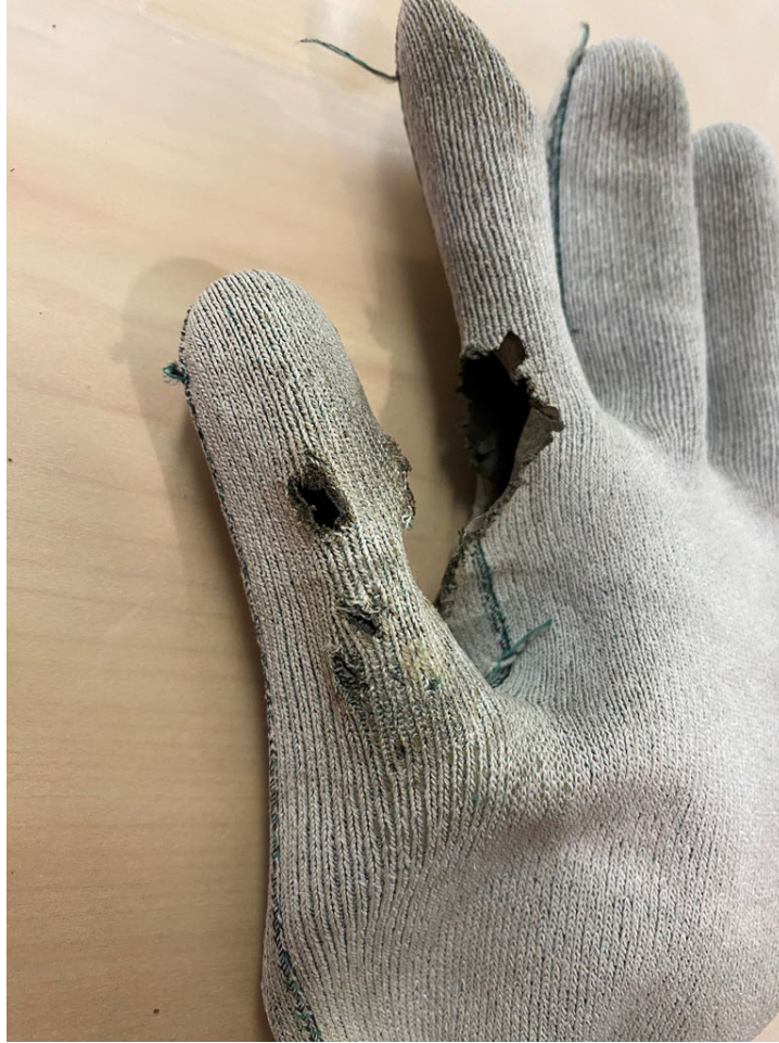
Figure F-4: Close up of internal damage to the glove, showing multiple small holes and charring consistent with shock current and arcing along inside of thumb and index finger.
