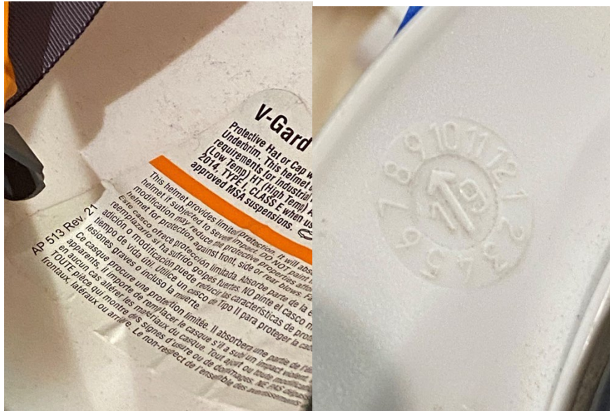
Figure F-17: Hard hat was of Class 1 Type E and was manufactured in 2019.
