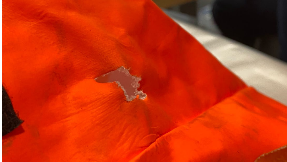
Figure F-12: Outside of left sleeve cuff there is a small open hole with minor heat shrinkage and wrinkling. Possible arcing point.
