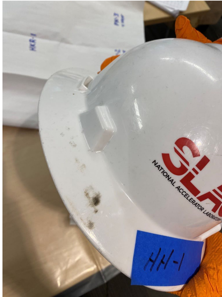
Figure F-16: Hard hat shows a possible soot deposit or heat damage mark. No residue will come off with rubbing.
