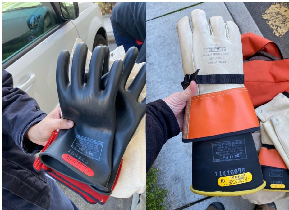
Figure 3-24: Class 0 (left) and Class 2 (right) sets of voltage gloves found in HVE1's work vehicle.
