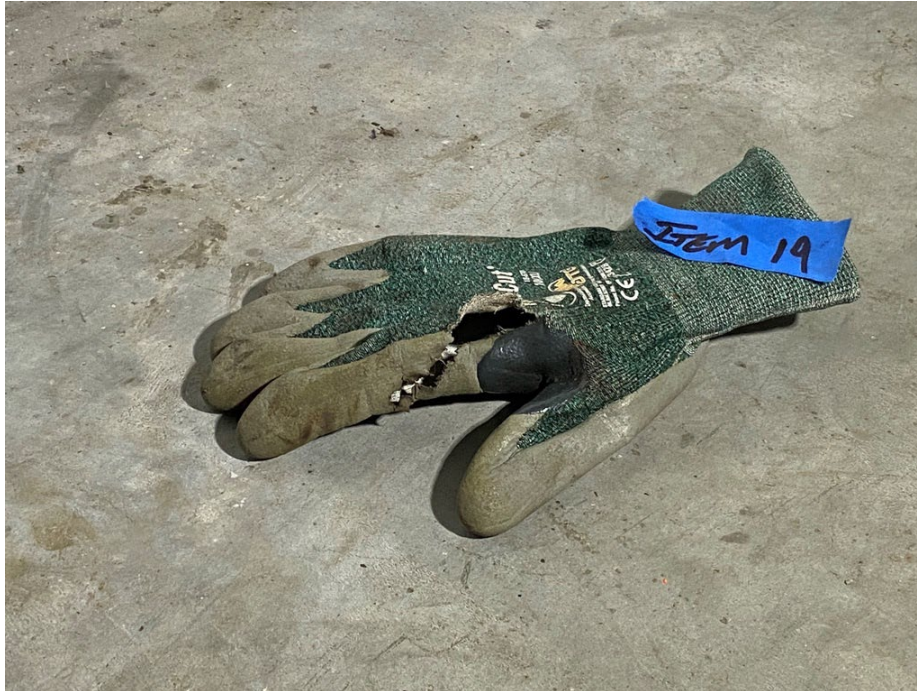
Figure F-2: Work glove turned out showing tear across index finger.
