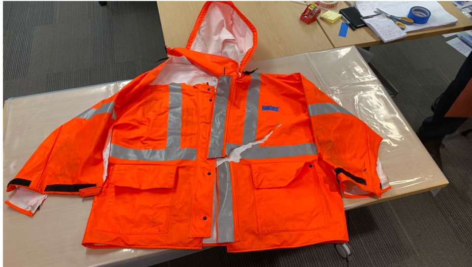
Figure F-10: Front of arc-rated high-visibility rain jacket with no sign of arc flash damage.
