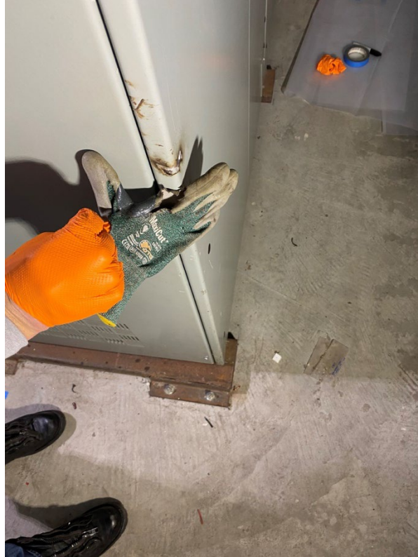
Figure E-16: Comparison of glove damage to the shock contact area for right hand.
