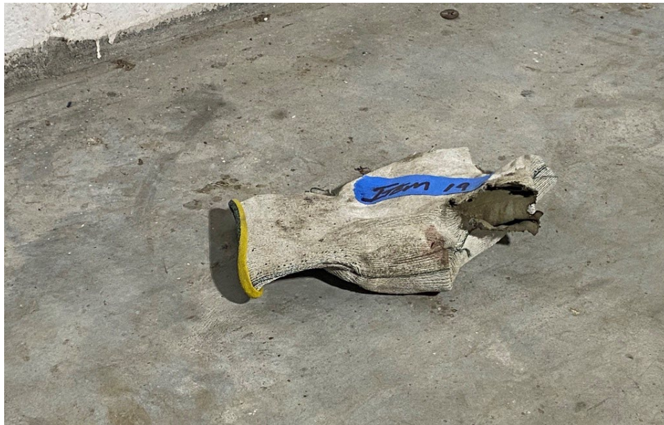
Figure F-1: Work glove was found turned inside out in Building 626, showing tears in the web of the thumb and index finger.
