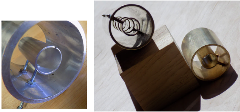
Figure 2: Photographs (with ends removed for visibility) of a single cell, on the left, along with a 4-cell longitudinal, split-cylinder polarimeter, on the right.
