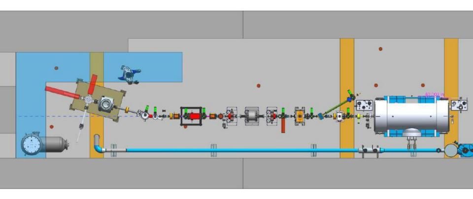
Cryo lines hug the wall, waveguides on same side as cryo lines Heat exchanger added to the mix, Rao says this will make things more efficient and stable
