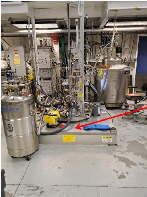
Figure 2.10: The dilution refrigerator. The left side shows the top of the DF with the TC mounted on top. Most of the DF was located in the pit below aluminum safety plate. On the right is a schematic of the DF's components in the pit [16].
