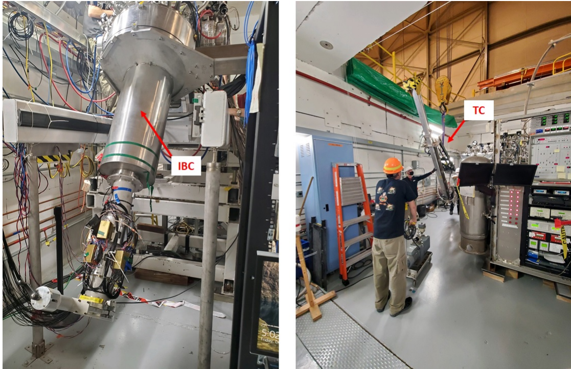
Figure 4.12: Target loading at the UITF. The left shows the IBC as it was being rotated vertically for loading. The right shows the UITF ceiling tiles removed allowing the TC to be attached to the crane, lifted, and mounted to the vertical IBC.
