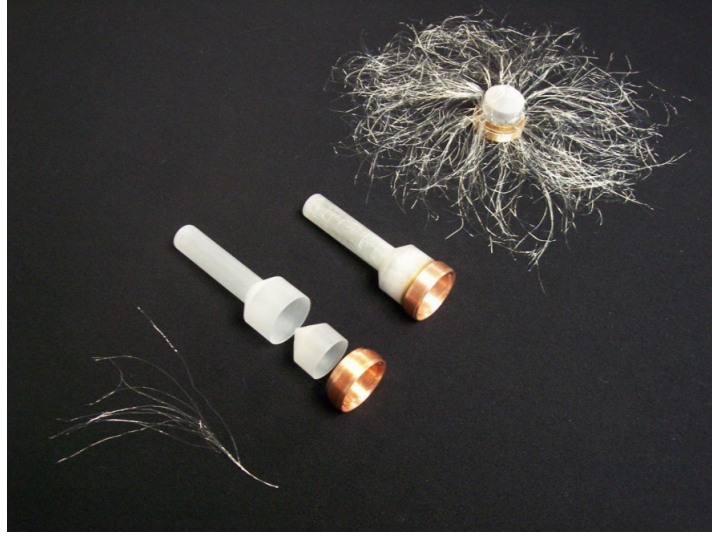
Figure 2.2: Layout of the HDice target cell used during g14. From left to right, a bundle consisting of 14 Al wires, a sectional view of the Kel-F pieces that attach to the ring, a completed target cell, and a target cell after 60 bundles are soldered and the wires separated to be positioned.
