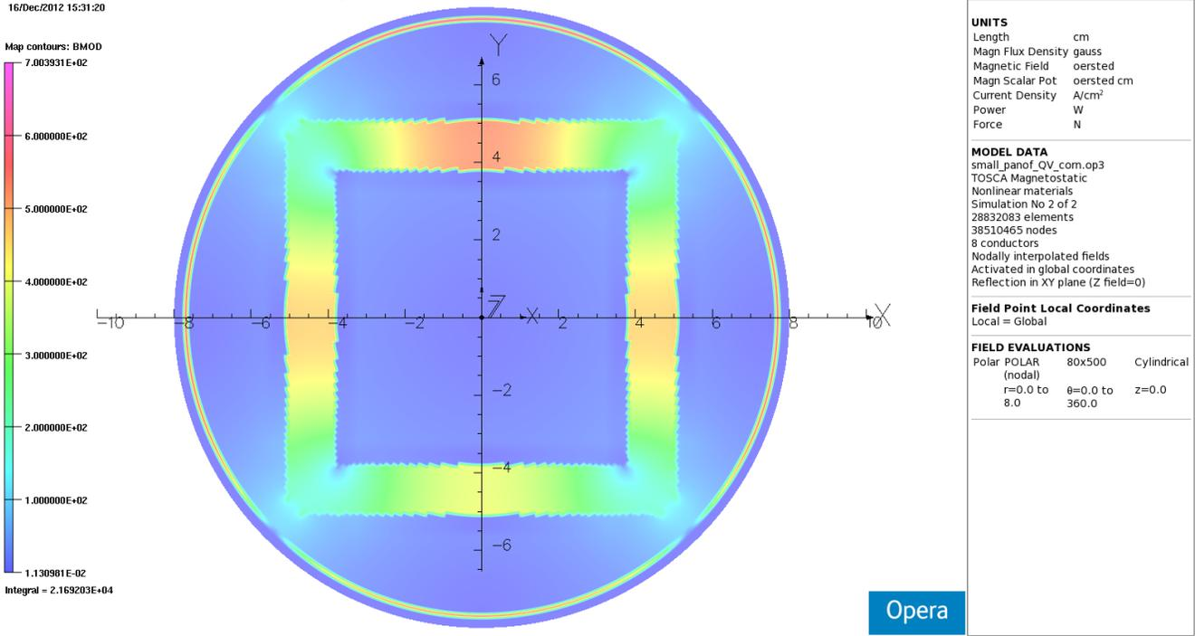
Figure 15. BMOD in the midplane. One sees peak field about 700G in the mu-metal shell and perhaps 500G in the core rods. It follows that one can get a lot more deflection and focusing out of this unit than the FEL gun requires. I over-design. Core is only 7.83mm wide at the flats on the 1/2" rods but peak flux is similar.
