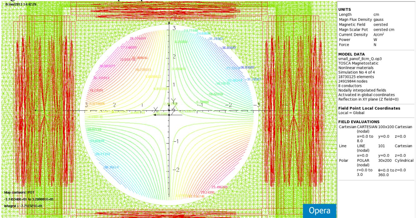
Figure 24. Potential lines for combined quad and dipole. The pattern moves down uniformly.
