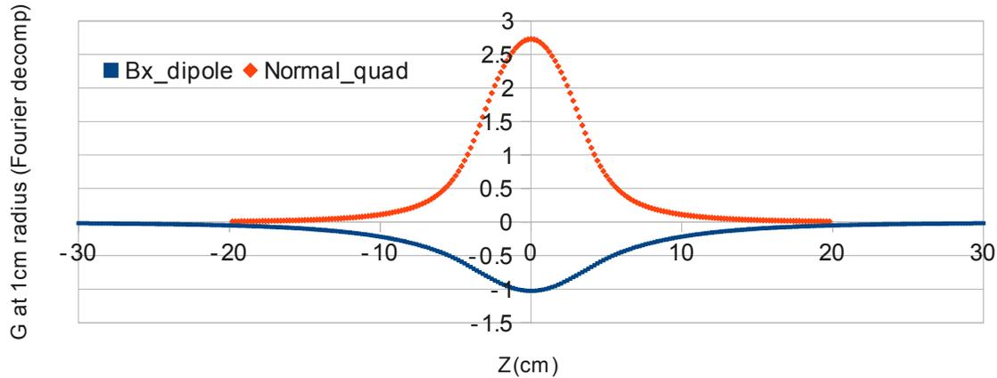
Figure 3. Fourier components of model in figure 4 with 460 AT in quad and 15 AT in dipole. 1 cm radius
