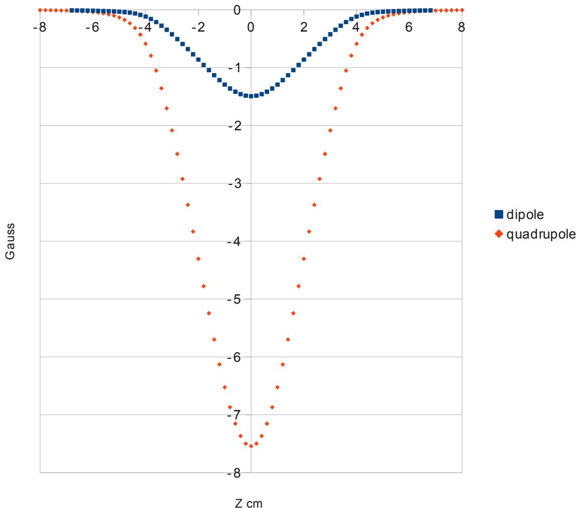
Figure 25. Plot of dipole and quadrupole components for the 8cm long combined function magnet. Compare with figure 16 on page 10, the same plot for the 10cm long unit.
