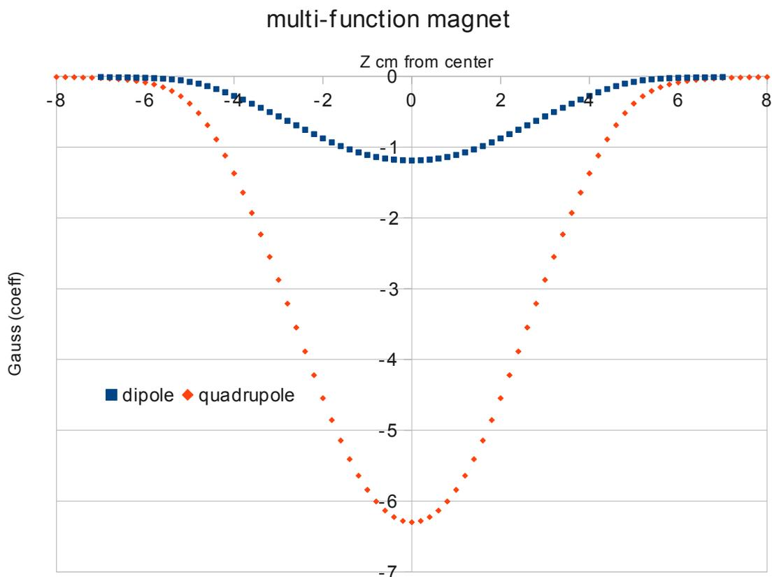
Figure 16. Multipole coefficients as a function of Z for the model. Integrals at top of page. Field clamp annular plate extends  $z=[4.85,5]$  cm and has a hole radius of 3.2 cm. Nothing to be seen on this scale at 1.6 cm beyond the plate. There would be if the dipole field were higher.
