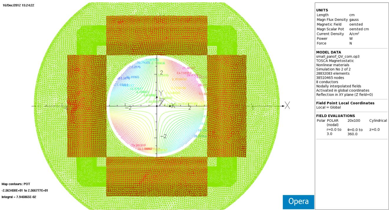
Figure 14. Potential lines. The quadrupole pattern is not centered because both quad (35G integral) and dipole (7 G-cm integral) coils are excited. One sees the 1mm mesh used throughout the magnetic material and the air containing the coils too.
