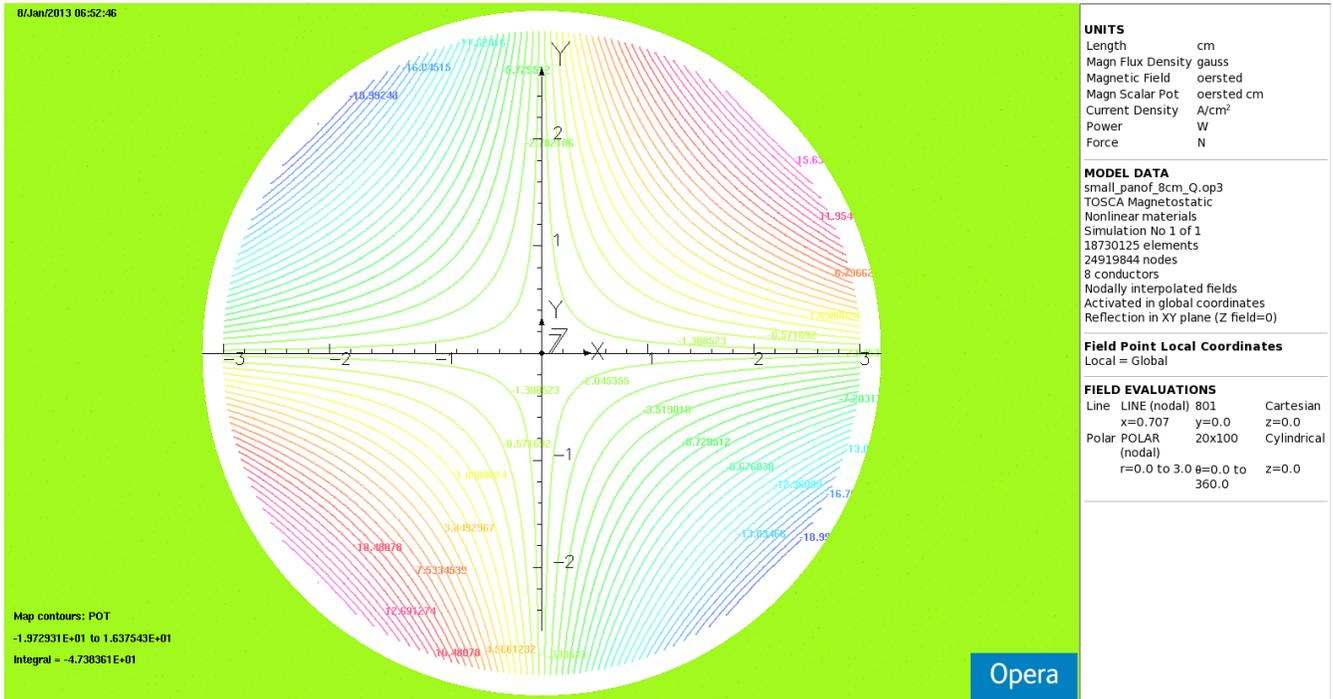
Figure 23. Potential lines of pure quad in 8cm combined function unit.
