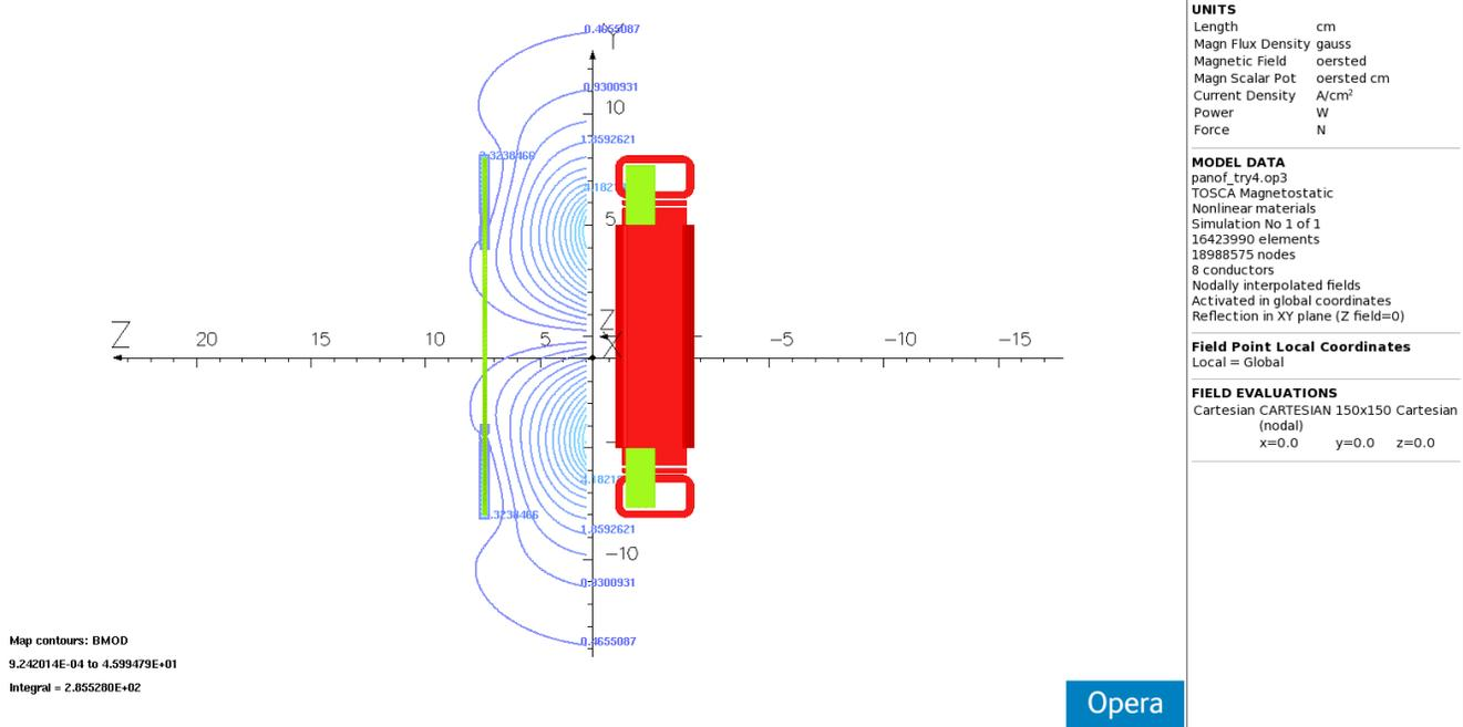
Figure 8. Same BMOD plot as figure 7. Most of the 100 field lines wrap around the magnetic material near  $z=7.4$ .
