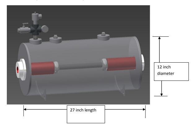
The tank is not a "Pressure Vessel" since it is protected from over-pressure with an ASME section IV rated pressure relief valve. Our tank will also be fitted with a compound gauge that can monitor the tank during pump-down, pressurization, and sealed storage.
