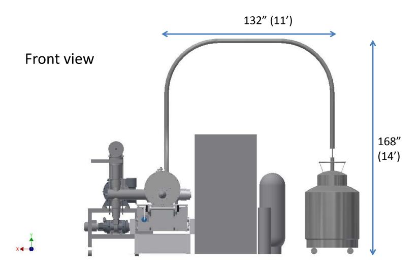
Additional 6" height is also needed to support the arch.
