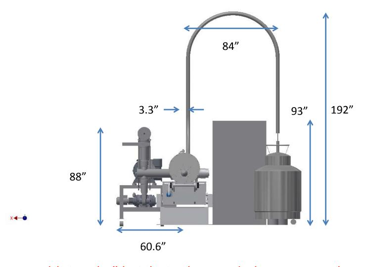
Additional 6" height is also needed to support the arch.
