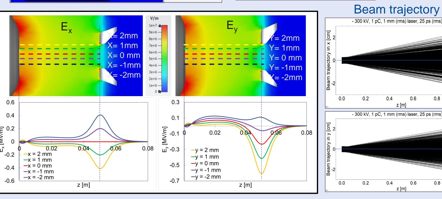
GPT simulations with the modified gun for the magnetized (0.075 T at the cathode) and non-magnetized (0 T at the cathode) beam
