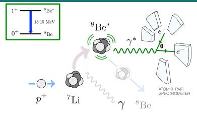
1.04 MeV proton beam on  $^7Li$  to  $^8Be(18.15) + \gamma$ . Followed by decay. Looked at  $e^{\pm}$  pairs from internal conversion.
