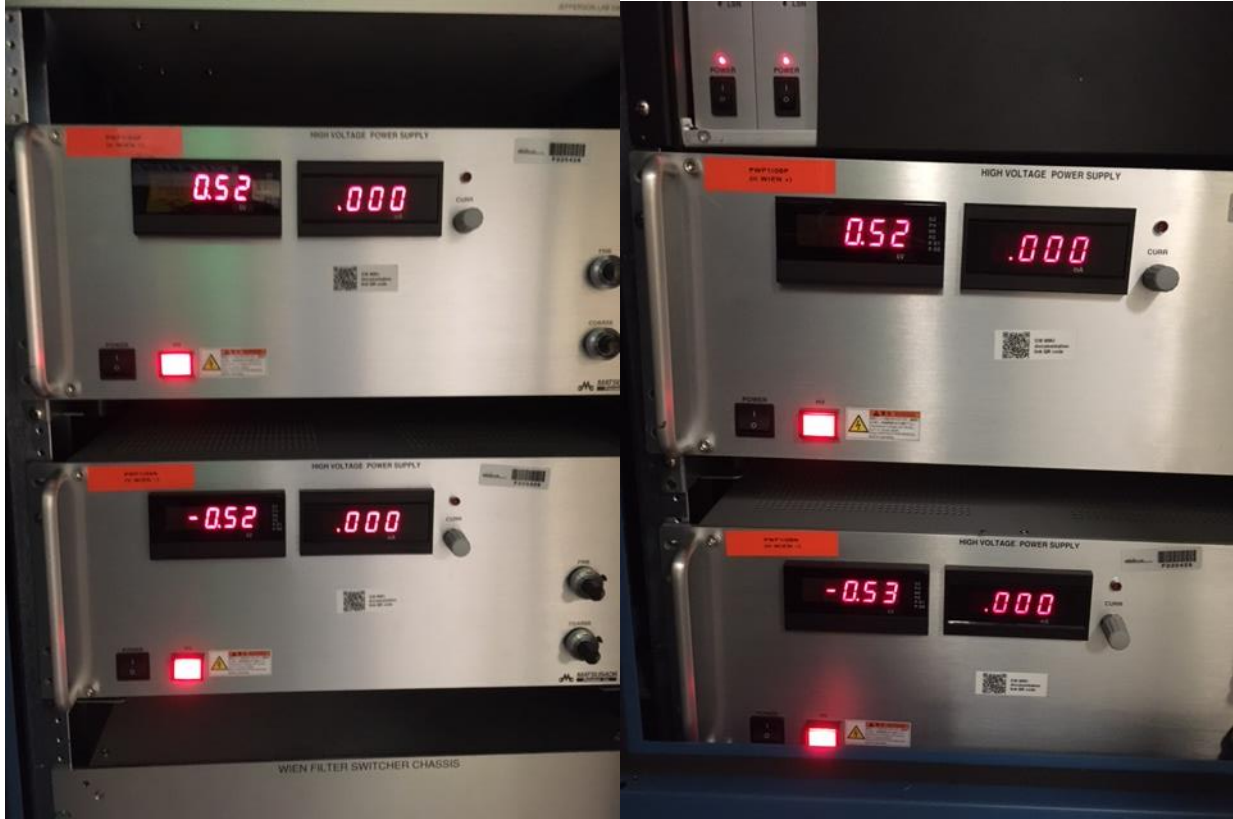
Figure 6. LEFT: Vertical Wien filter HV system (top stack). RIGHT: Horizontal Wien filter HV system. The pictures show how the systems should look like when powered, high voltage enabled (toggle switch illuminated in red), and 500 V Set point. Notice the lower power supplies display negative values, these correspond to the negative power supplies.
