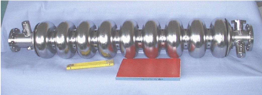
Figure 5.16: The TESLA style 9-cell niobium cavity.
