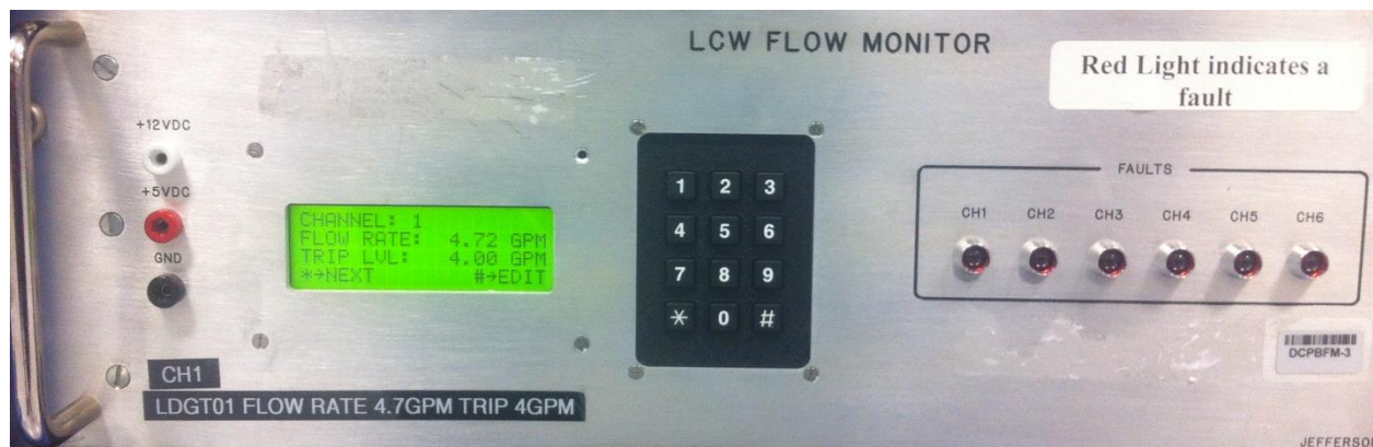
Figure 4: Cathode magnet LCW flow rate monitor chassis at the GTS mezzanine in Rack GL01B05. The status of this interlock is displayed in the control screen under “Solenoid LCW”.
