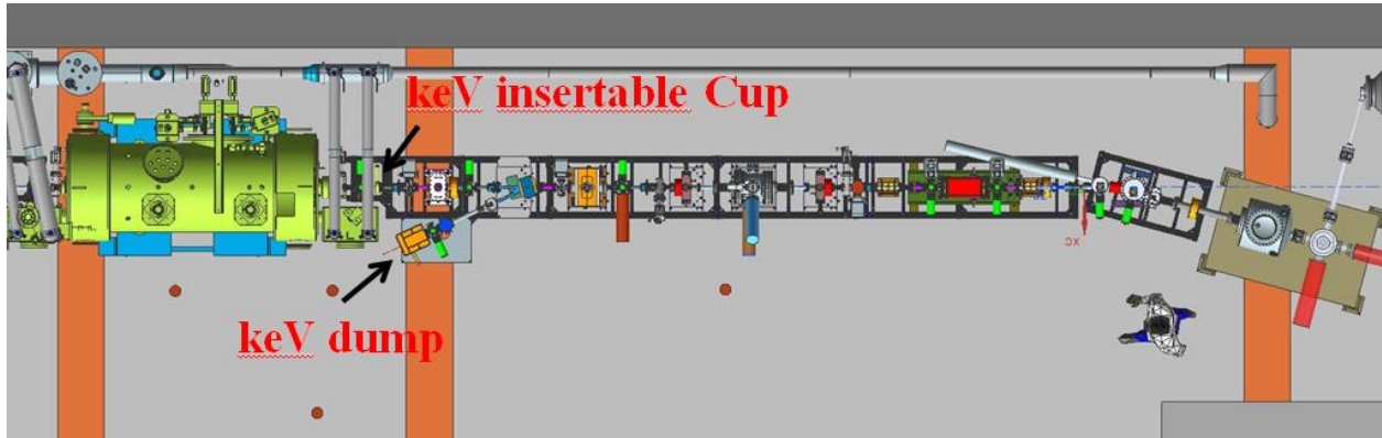
Figure 10 keV beam line top views. The figure shows the location of the 1/4 Cryomodule, the keV fixed dump, and the keV insertable Faraday Cup
