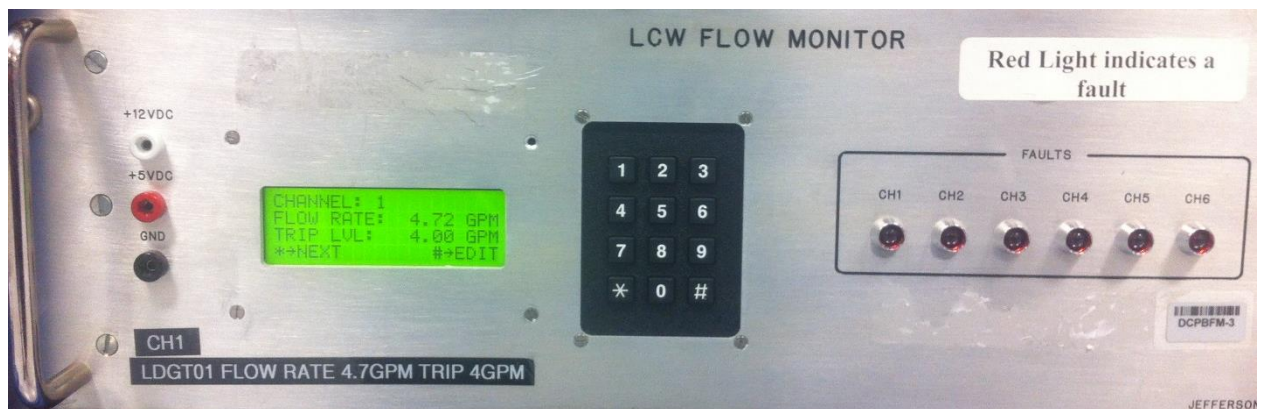
Figure 4: Cathode magnet LCW flow rate monitor chassis at the GTS mezzanine in Rack GL01B05. The status of this interlock is displayed in the control screen under “Solenoid LCW”.
