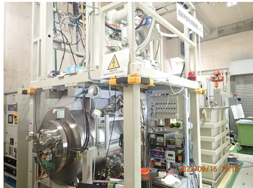
40 kV, 300 kW electron beam heating machine @ NIFS
