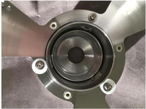
The overall length of the anode assembly was measured at 2.235". The sum of the measured individual pieces came to 2.226". This needs to be confirmed with assembly drawings (task for Carlos: ask Shaun for assembly drawing).
