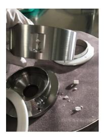
The existing screws are too long if the back ceramic ring is removed for grounding the tube.
