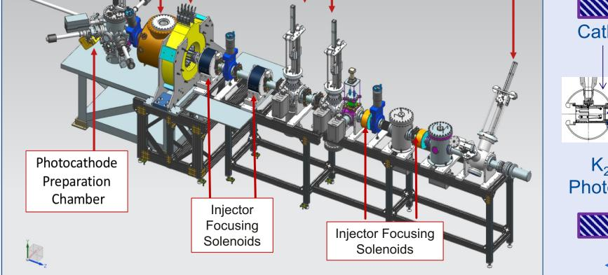
Gun Test Stand consists of a K<sub>2</sub>CsSb photocathode preparation chamber, DC high-voltage photogun operating at -300 kV, cathode solenoid magnet to magnetize the beam, and a beamline with two YAG screen-slit combinations at 0.5 m and 2.0 m, a YAG-screen at 3.75 m, four injector focusing solenoids, steering magnets, harp, and beam dump.
