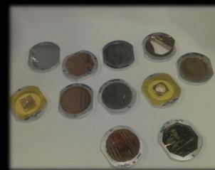
[Above] Foils used in polarimeter. Usually gold, silver, or copper. Range in thickness from .01 μm to about 10 μm. [Left] Scattering angle as a function of thickness for the three methods of calculating angle.
