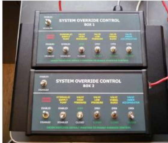
Figure 6: System Override Box
