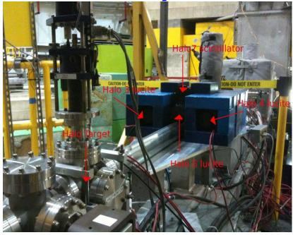
Halo target: thin aluminum with two holes, mounted near usual Hall C pivot on superharp linear drive mechanism
