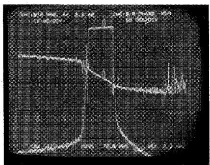
Fig. 12. The SO of Fig. 11 with a three-section 140-MHz filter connected to the input.
