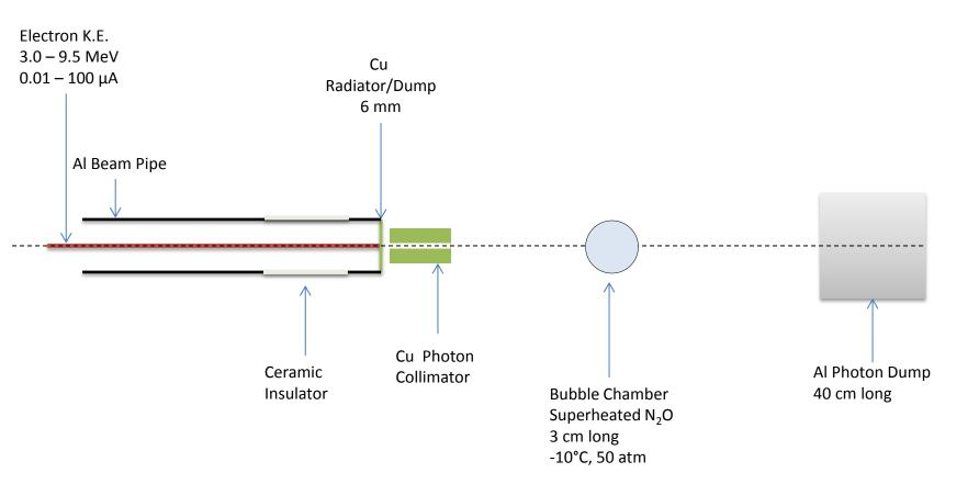
Large Dynamic Range Diagnostic Station (LDRDS) was installed in 5D line for beam test in Spring and Summer ➤ Remove before Bubble Chamber installation
