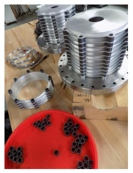
The Cavities have been tuned to their target frequency 2.774 GHz by precision grinding the Silicon Carbide spacers that separate the cavities segments.
