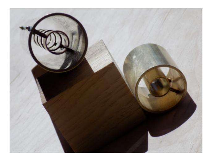
The assembly technique works well, the components remained coaxial. The single resonator has been RF tested, and to our surprise it resonates at 2.5 GHz rather than the target of 2.7445 GHz. Although we missed the frequency, RF testing these prototypes will tell us a lot about coupling to the resonance as well as the coupling between resonators in the four split ring prototype.
