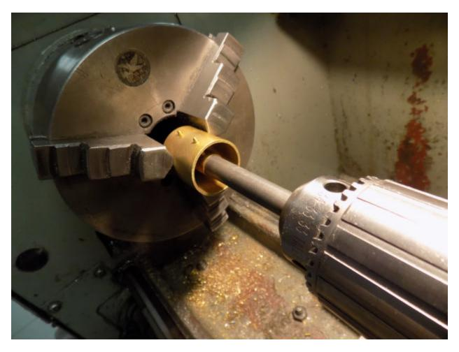
The single resonator components were then fixtured and soldered in a lathe because it has two co-axial chucks. The four resonator assembly was similarly fixtured after putting it together like a ship in a bottle.
