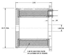
Figure 2: Diagram of the solenoid magnet fabricated.
