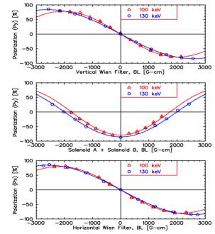
Figure 6: Variation of the electron polarization as a function of the magnetic integral for each spin rotator is shown. The two calibrations used different photocathodes, which explain the difference in maximum polarization.
