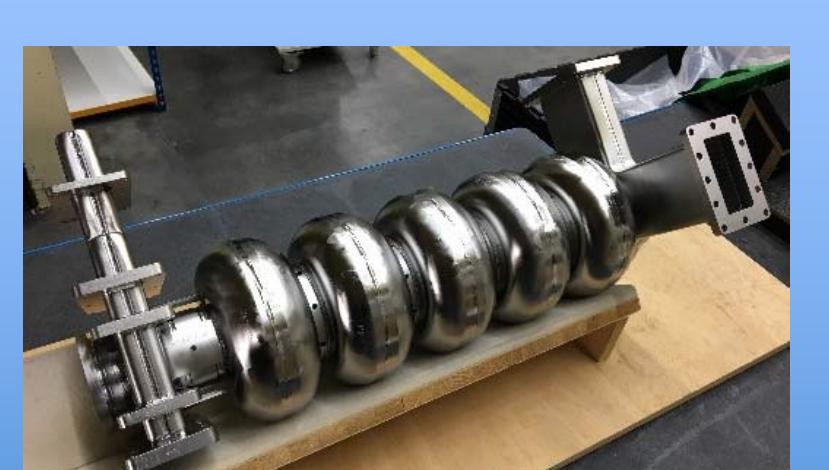
2 Low energy beam line with compresses 60 psec bunches to ~few psec for acceleration
