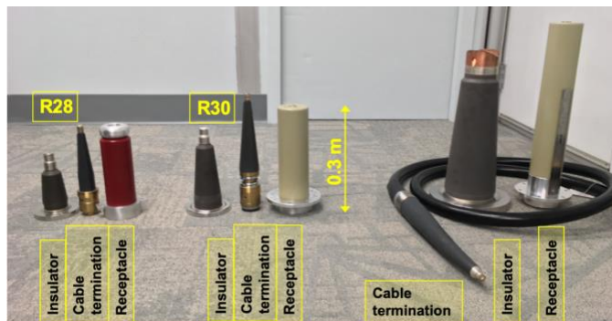
Fig. 1. Doped alumina conical insulators, cable terminations and epoxy receptacles utilized at JLab for various photoguns. Left: Insulator and R28 cable termination for the 100 and 200 kV photoguns. Center: Insulator and R30 cable termination utilized in the 300 kV photogun. Right: The 350 kV rated cable termination is utilized to connect the photoguns to their corresponding power supply via the shown epoxy receptacle. The large insulator was custom made for a different R&D program and thus is not compatible with commercial high voltage terminations.
