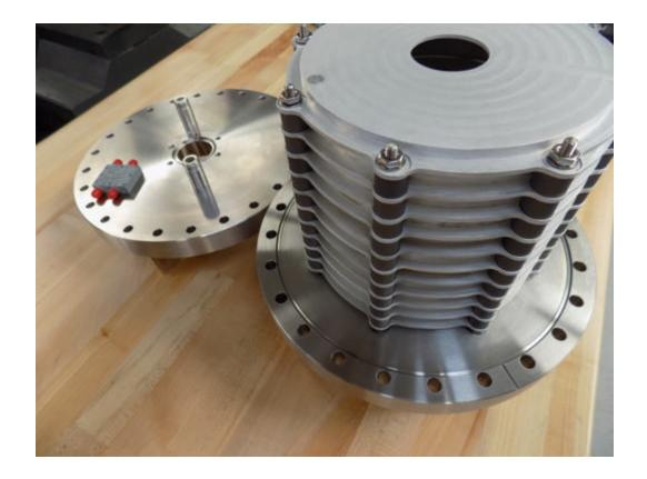
Not complete: need to trim cavity to tune its frequency of operation, build its antennas, and build a down converter from 2.7445 GHz to 249.5 MHz for VQ detection.
