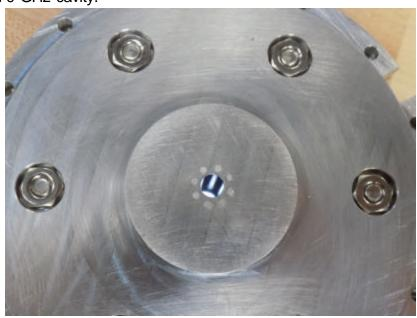
The TE011 mode shifted frequency by 10 MHz or so, but the operation of the mode seemed unaffected by the rods. The purpose for this modification was to try and reduce the coupling of the charge signal into the cavity, or the excitation of the resonance by a slanted beam. Experimentation with driving this mode with external antennas seems to indicate that one can still drive the mode with a slanted antenna, so while interesting it does not immediately appear to be a solution.
