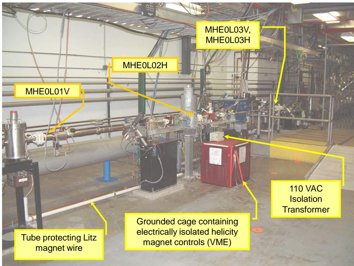
Figure 1: Helicity magnets control crate in CEBAF injector.
