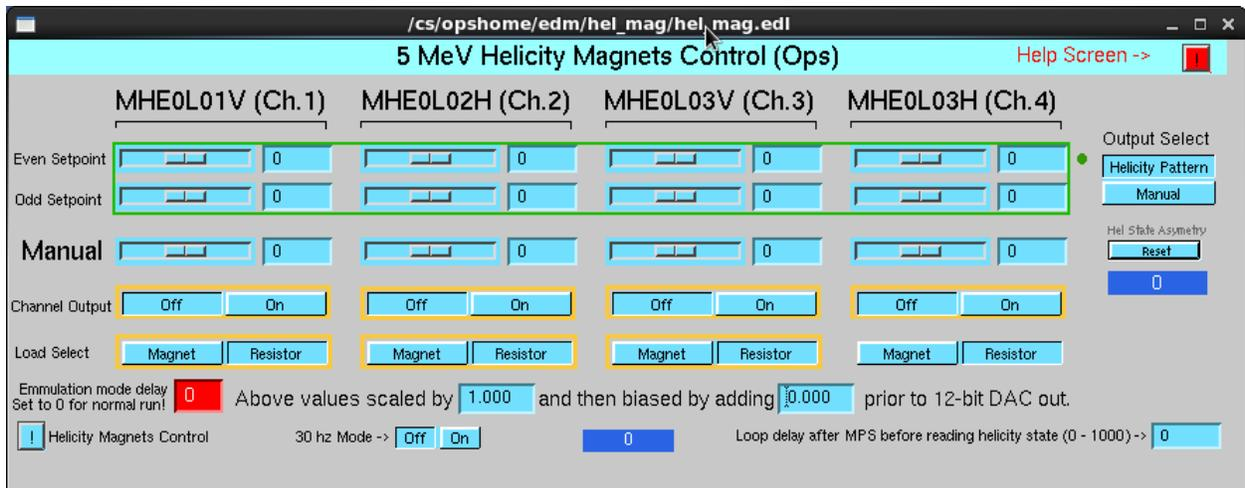
Figure 2: Helicity magnets control screen. For the upgrade, the “Manual Mode” will be used, too. The 30 Hz Mode was used as a PZT booster system to measure adiabatic damping in the Injector. This system is not in use anymore. FOPT system will be used instead.
