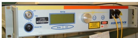
(a typical fiber laser amplifier)
