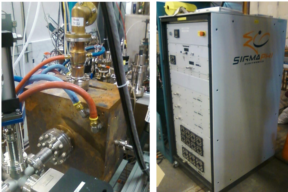
Figure 1: (left) the normal-conducting copper-cavity 748.5 MHz buncher installed on the UITF keV beamline, and (right) the 7 kW solid state amplifier located above Cave 1 near the electronics racks. A rigid coaxial waveguide connects the two devices, with the waveguide passing through a penetration in the Cave 1 roof.
