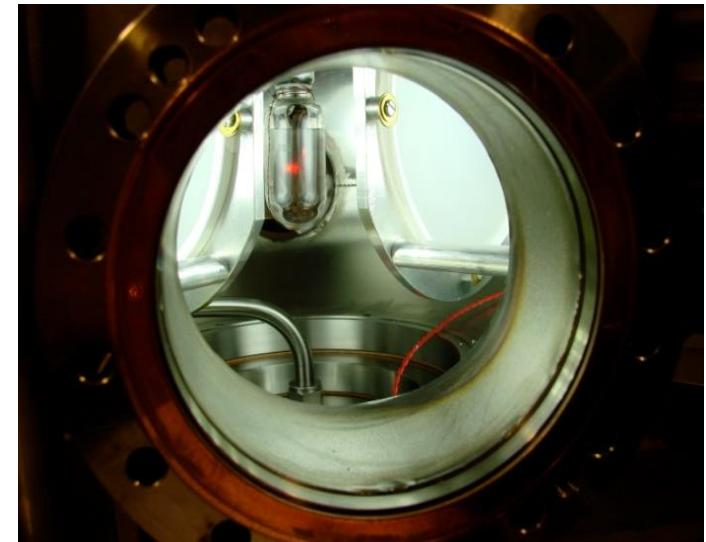
$\text{C}_4\text{F}_{10}$  Bubble Chamber
