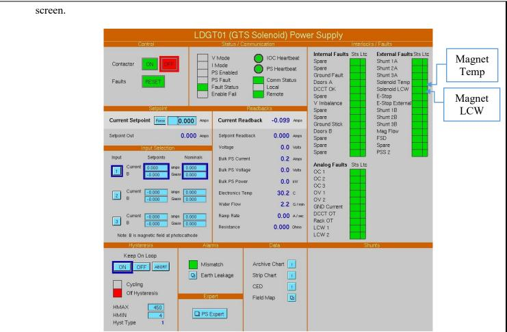
*Figure 6: Cathode Solenoid power supply control screen. The firmware is under iocfel12 in Rack GL01B02.*
