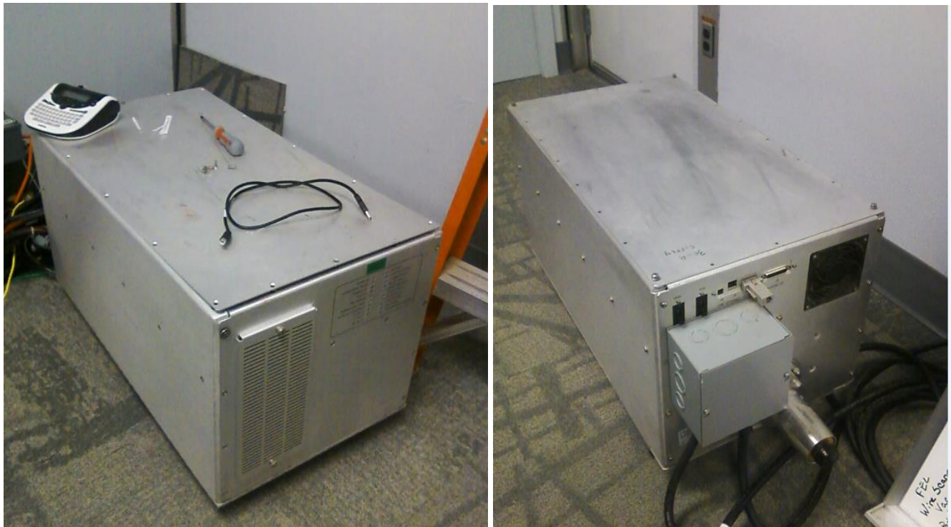
Figure 4: The 225 kV Spellman high voltage power supply, front (left) and back (right), will be located inside the UITF enclosure placed near the photogun, and operated remotely from the UITF Control Room. A high voltage cable connects the photogun to the high voltage power supply, there is no exposed high voltage and no SF6 tank required.
