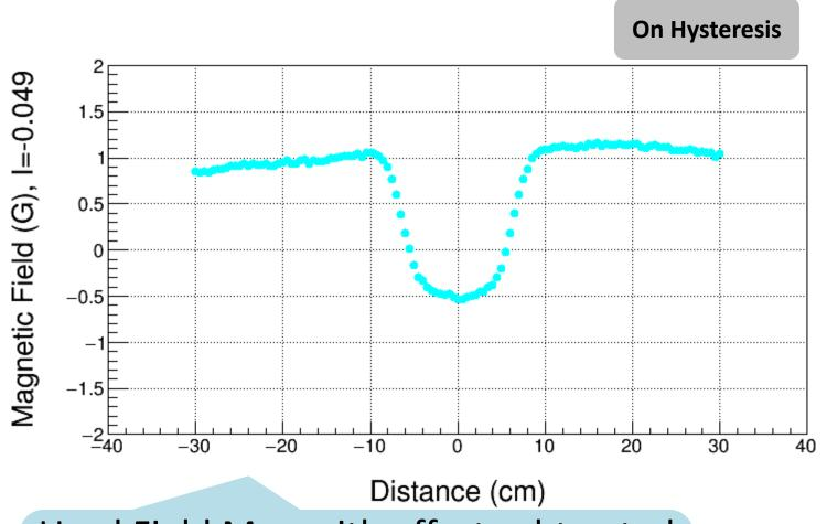
Used Field Map with offset subtracted to find 0 BdL BdL = 43 G-cm - Offset ~ 0
