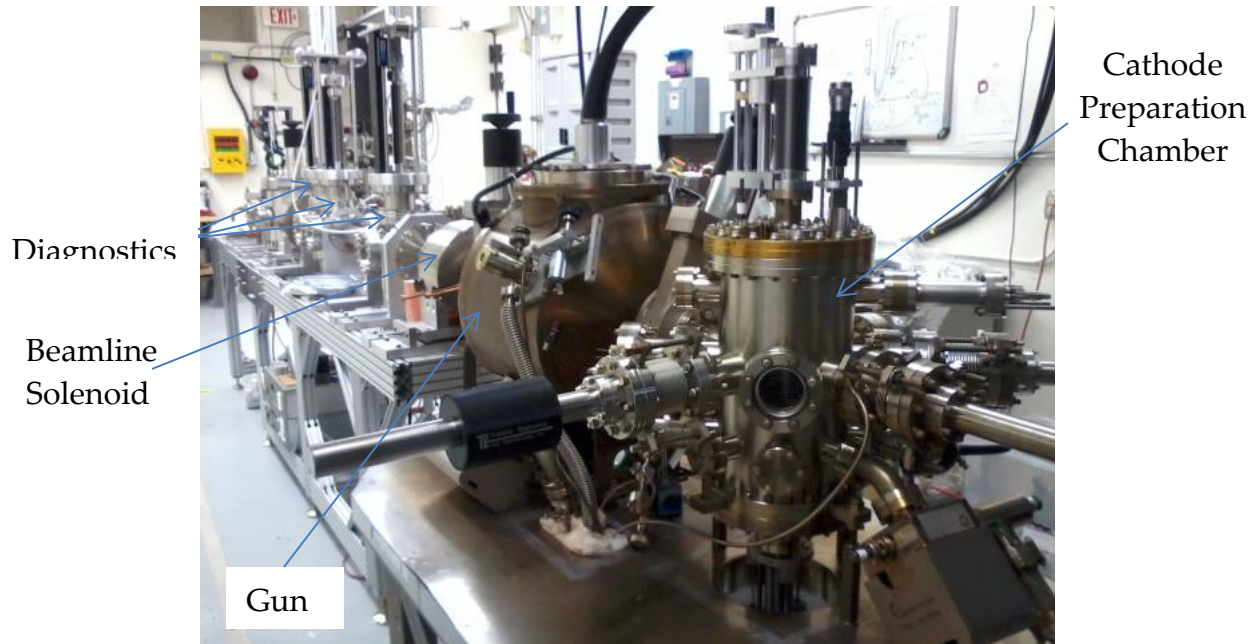
Figure 2: Preparation chamber, gun and beamline
