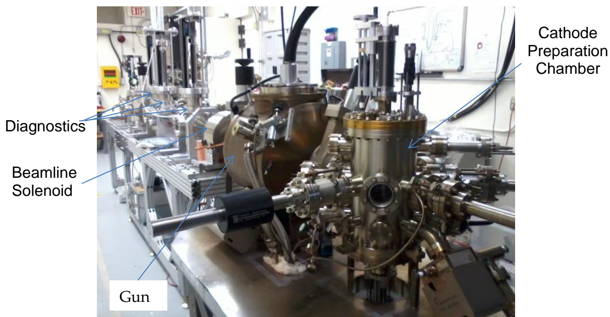
Figure 8: Preparation chamber, gun and beamline in the GTS.
