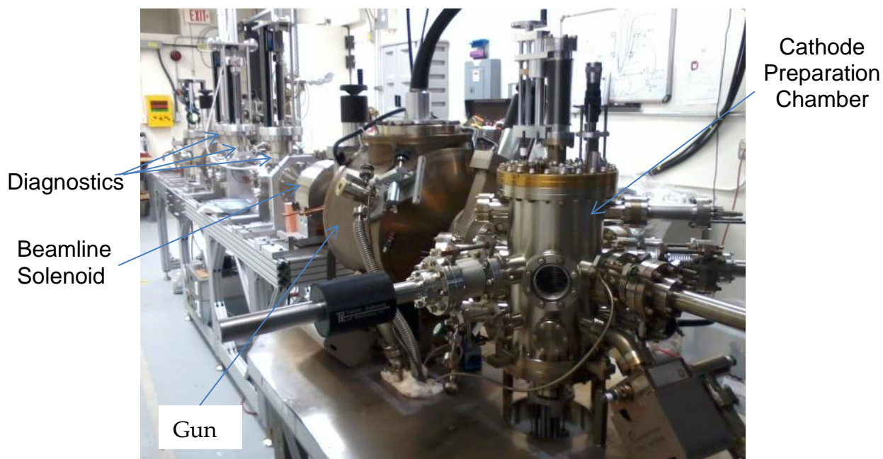
Figure 7: Preparation chamber, gun and beamline in the GTS.
