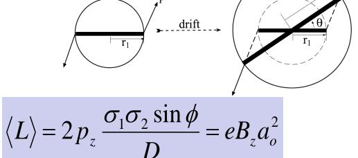
Angular rotation φ is measured from beam image at Cross 2 when multislit is inserted at Cross 1
